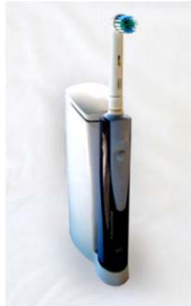
Rechargeable Toothbrush with an inductive charger (Public Domain Image courtesy Jonas Bergsten)
