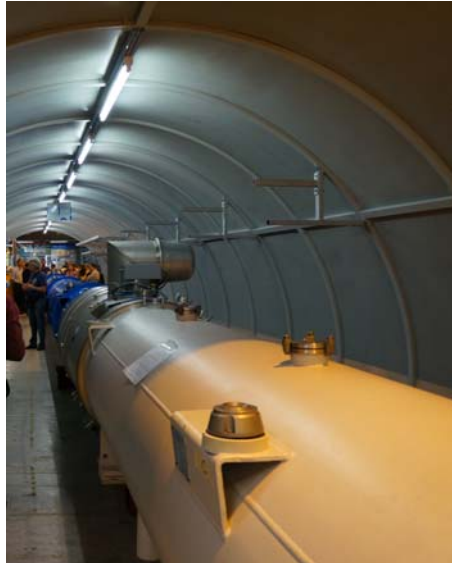
Beam magnet and Section of the Beam Pipe of the LHC. This section is actually no longer used and is in a service area 100 m above the operating LHC. The people you see are part of a BYU-I Physics Department Tour of the facility.
