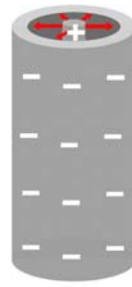
Oppositely Charged Coaxial Cylinders
