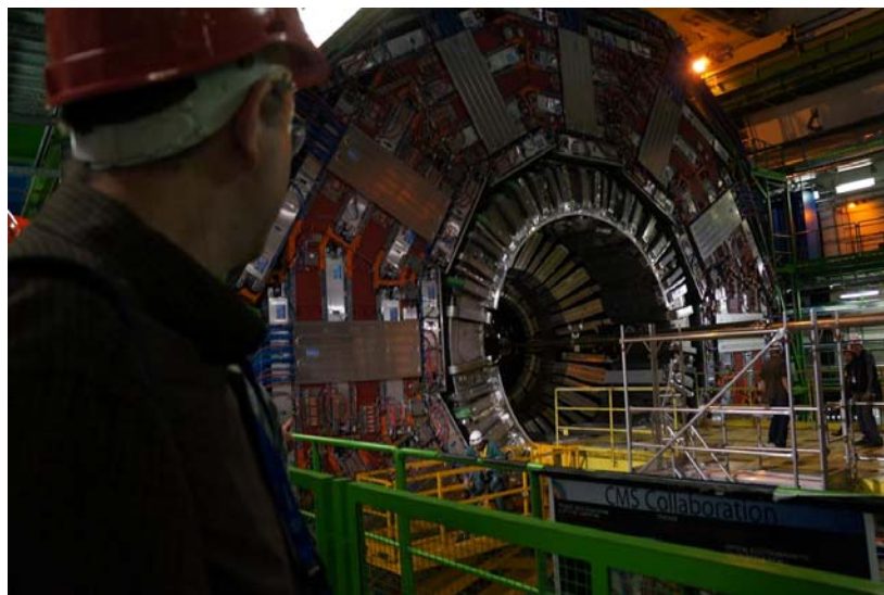
CMS Detector at CERN. The detector is constructed of a very large solenoid to bend the path of the charge particles.
