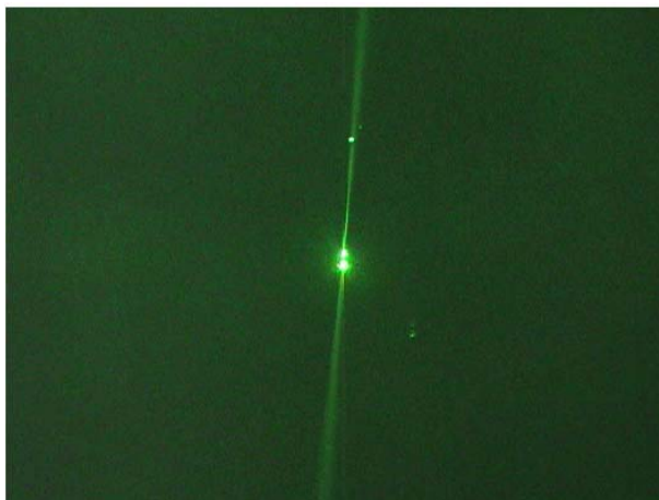
Figure 33.8. Laser Levitation (Skigh Lewis, Larry Baxter, Justin Peatross (BYU), Laser Levitation: Determination of Particle Reactivity, ACERC Conference Presentation, February 17, 2005)
