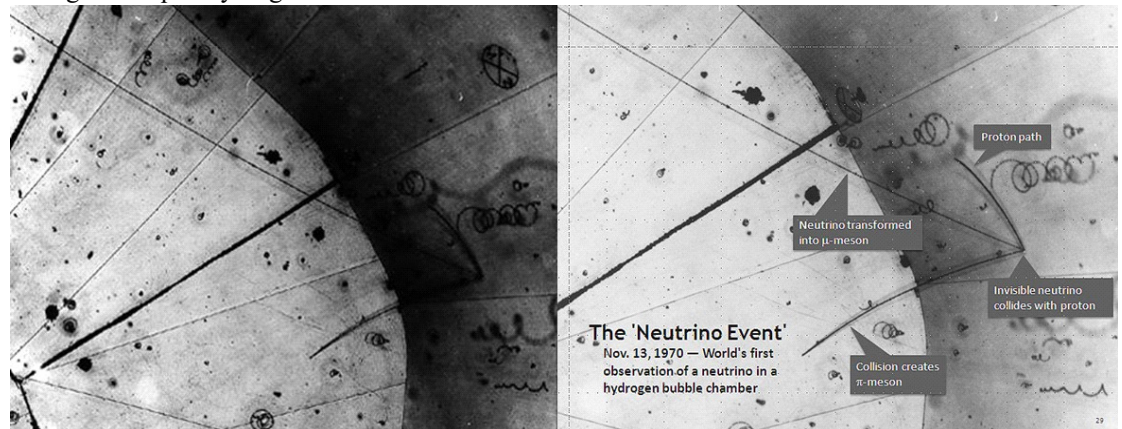
The first use of a hydrogen bubble chamber to detect neutrinos, on November 13, 1970. A neutrino hit a proton in a hydrogen atom. The collision occurred at the point where three tracks emanate on the right of the photograph. Image courtesy of Argonne National Laboratory.
