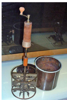
Joule Apparatus (Image in the Public Domain courtesy Gaius Cornelius)
