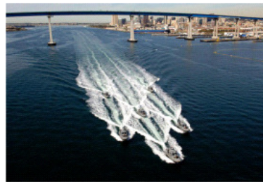
Boat wakes as a Doppler cone. Image courtesy US Navy. Image is in the Public Domain.
