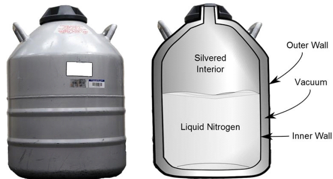
Figure 29.4. You might see our liquid nitrogen dewar in demonstrations. The flask is pictured on the left, and a schematic diagram of how a dewar works is given on the right.
