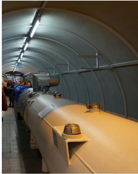
Beam magnet and Section of the Beam Pipe of the LHC. This section is actually no longer used and is in a service area 100 m above the operating LHC. The people you see are part of a BYU-I Physics Department Tour of the facility.
