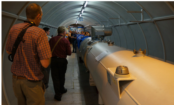
Turning magnets at CERN. This is an actual magnet, but this magnet is at ground level in the testing facility. The tunnel is a mock-up of what the actual beam tunnel looks like.
